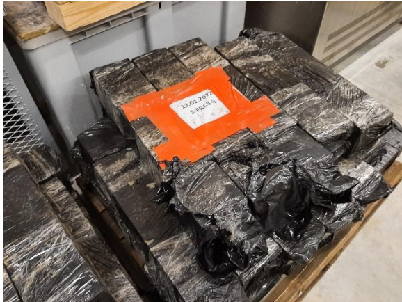
Figure 4 Beam specimens watered and covered with plastic sheet
